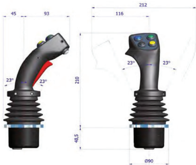
JHM base with MG type handle Complete code: JHM L4D/ANH-MG A4P9 R1P9
